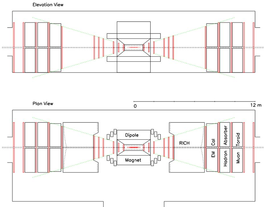
Figure 9: The BTeV detector layout.
