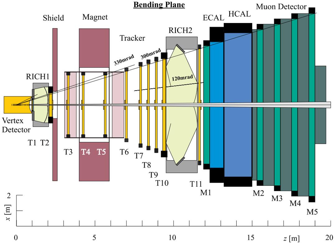
Figure 8: The LHCb detector layout.
