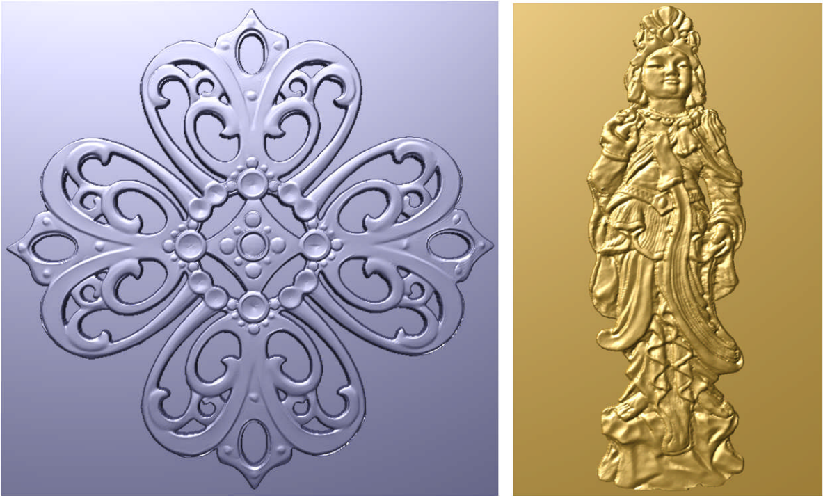
Fig. 6: An ornament bas relief (left) generated with the range domain method. The bas relief of the Malaysia Statue (right) is generated with the gradient domain approach.
