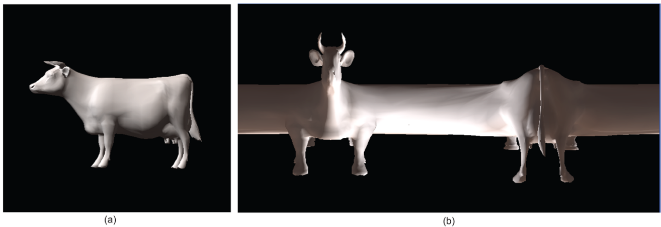
Fig. 6 Real-time rendering of 360 degree panoramas using GLC rasterization. (a) A perspective image of a cow model that consists of 5800 triangles. (b) Our panoramic rendering of the cow model at 47 fps at an 800 \times 600 resolution
