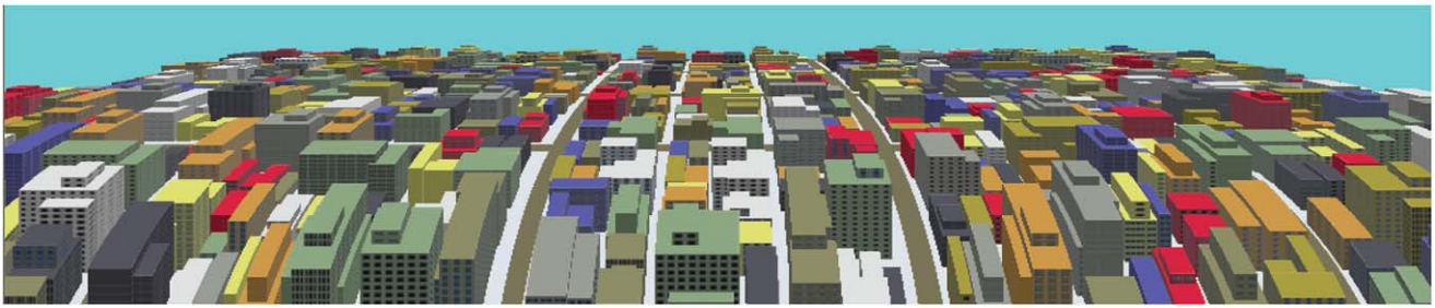
Fig. 1 Our framework interactively renders a complex city scene of 15k triangles at 70 fps. A cross-slit camera is used to render the scene at an 1024 \times 320 resolution
