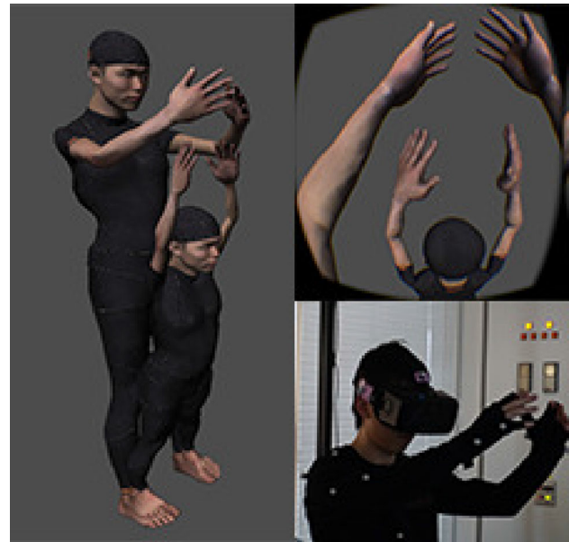
Fig. 1 Multi-embodiment (left), user view in HMD (top right), user wears HMD and motion capture (bottom right)
