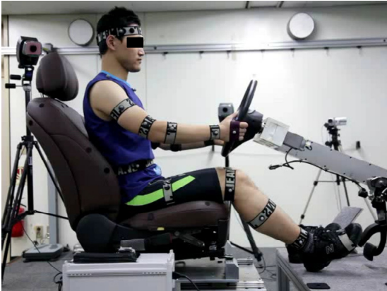
Figure 1. Measurement of driving postures using motion capture system
