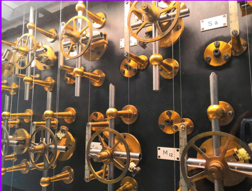
Doodson-Légé tide prediction machine, built in London in 1950. Photograph taken by H. M. Rawsthorne at NOC, Liverpool, on 15/01/2019; licensed under CC BY 4.0.
