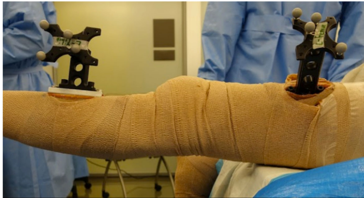
Fig. 1 Photograph demonstrating the arrays of reflective markers used for infrared motion capture analysis, which are fixed to the femur (right) and the tibia (left) using a combination of screw fixation and bone cement
