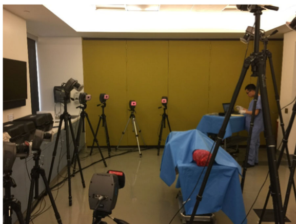
Fig. 2 Room set up for the measurements. An operating room (OR) table was positioned in the center of twelve motion analysis cameras on tripods at different heights and angles. These cameras were pre-calibrated prior to each measurement session
