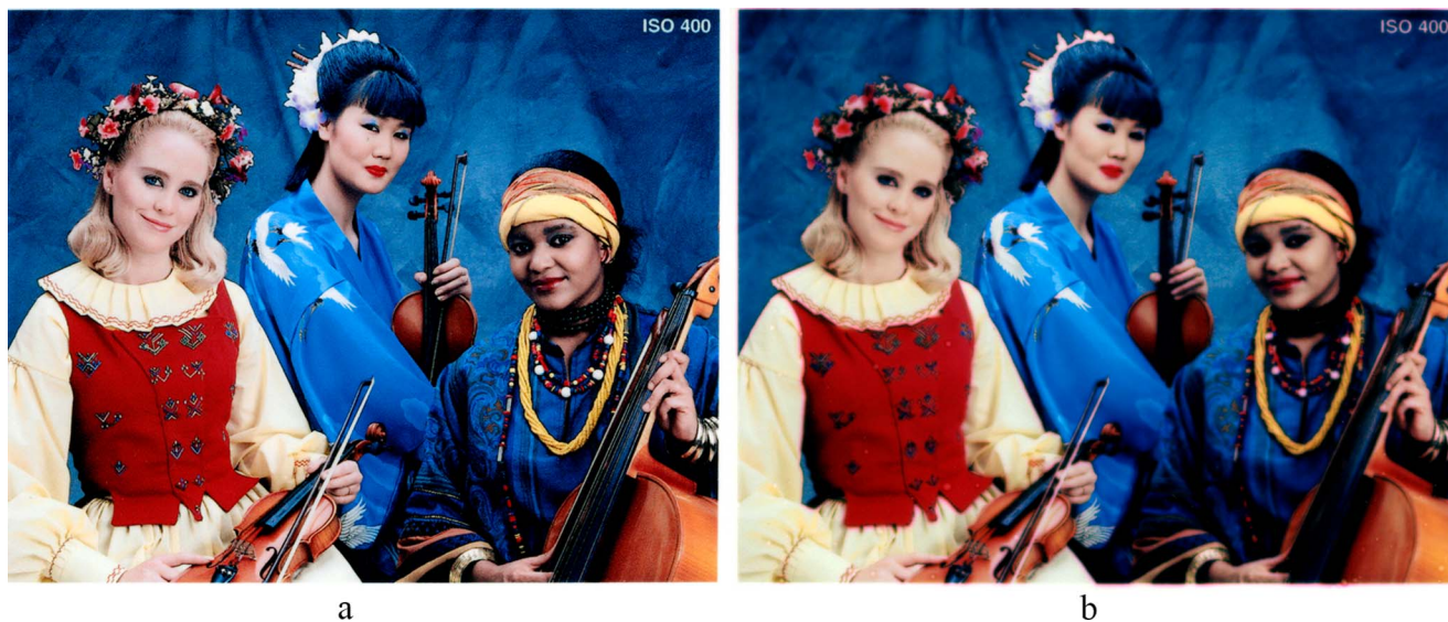
FIGURE 5. Inkjet prints showing examples of (a) the original print and (b) after dye migration. Images courtesy of the Image Permanence Institute.
