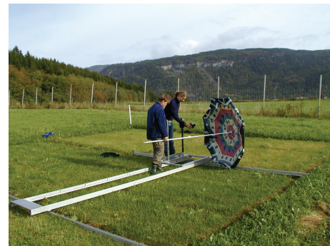
FIGURE 3: Positioned image acquisition to map the grass-clover sward.
