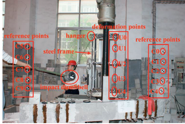
FIGURE 3: Impact test on a steel frame [28].
