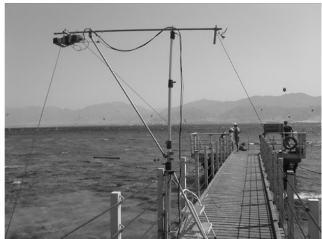
Fig. 1 The construction of the hyperspectral camera on the bridge. At this fully extended boom height, the camera can cover 3 × 6 m of reef
