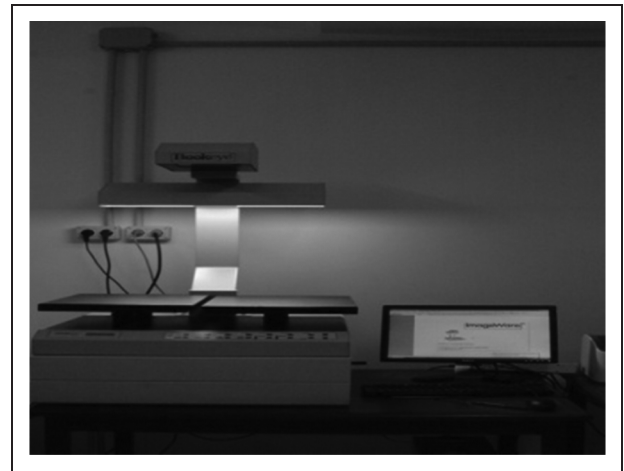
Picture 3. Book eye A2 scanner used in manuscripts and rare books digitization in 2008. Source: Field data, March 2015.
