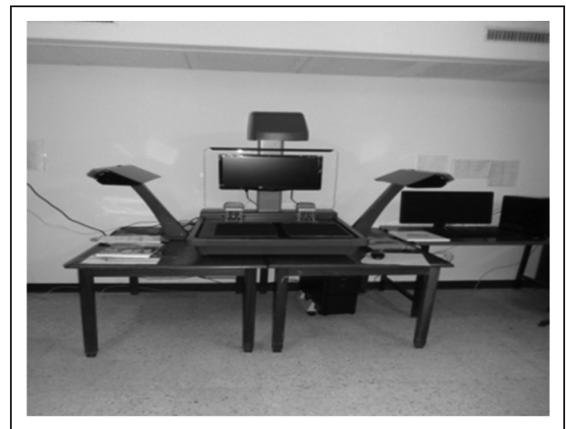
Picture 4. Copybook™ Onyx RGB scanner used in manuscripts and rare books digitization for urgent requests since 2012.
