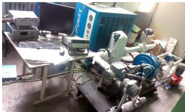
Fig. 1. single screw expander experimental system
