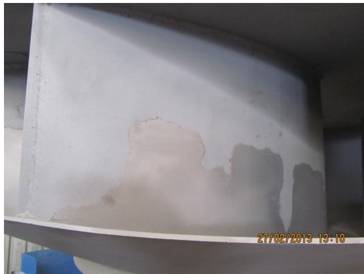
Figure 3. Final state of a rotor for a sugar production facility after a working campaign and protected with Cr and W cermet layers.
