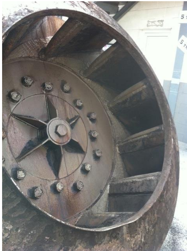
Figure 2 Final state after a working campaign of a rotor in a sugar production facility.
