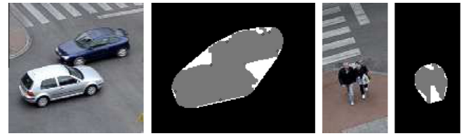
Fig. 10. Object occlusions and convex hull. The convex hull is represented in white and the foreground blob in gray color.
