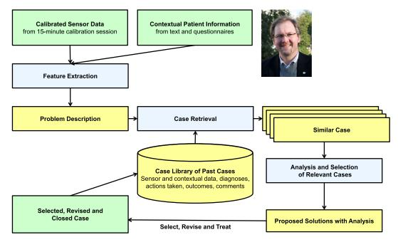
Fig. 5. Overview of the Mälardalen Stress System.
