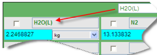
Figure 10. To obtain a higher heating value, de-select H 2 O and select H 2 O(L) from the products block and then press Super-Calculate to update all results.
