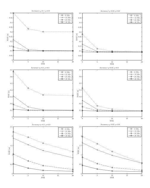
Figure 9: Localization accuracy for different wall reflection factors ( $\rho \in \{0, 0.5, 0.9\}$ ) as a function of the SNR and the number of microphones M. Each column presents results for different spatial resolutions (r = 0.1 and r = 0.01 m).
