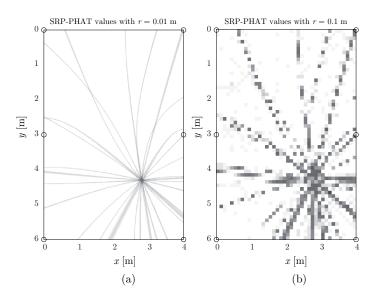
Figure 2: Accumulated SRP-PHAT values for a 2-D spatial grid (4  $\times$  6 m and M = 6 microphones) with different spatial resolutions. (a) r = 0.01 m. (b) r = 0.1 m.
