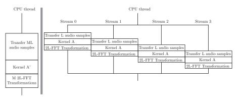
Figure A.2: Parallelization obtained with streams when M=4.
