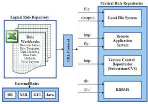
Fig. 3. Architecture of OpenRules (from http://openrules.com).
