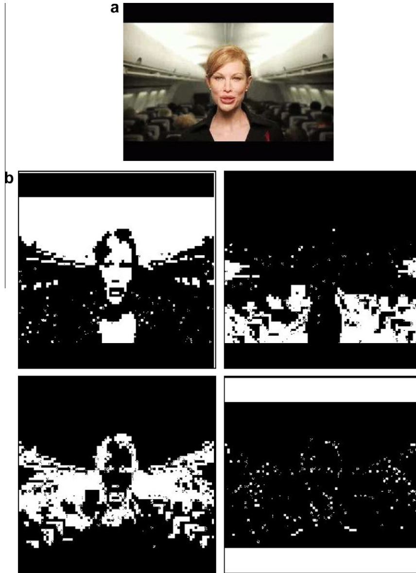
Fig. 11. Using K-means algorithm, pixels of original image, for example in (a), are clustered into four dominant groups according its color value. Then, four bitmaps, for example (b), are established to show the data distribution of pixels in each dominant groups.
