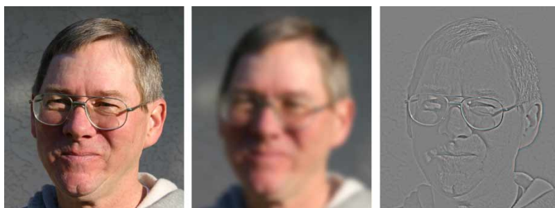
Figure 3. An image of a person (left), a low-pass filtered version of that image (center) and a high-pass filtered version (right). Copyright ©, 2005, Bahill, from http://www.sie.arizona.edu/sysengr/slides/ used with permission.
