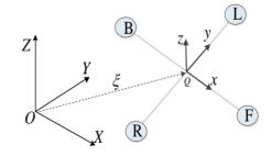
Figure 1. The definition of quadrotor's position coordinate system
