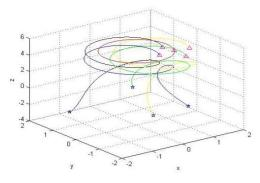
Figure 7. Simulation curve of quadrotor formation maneuver
