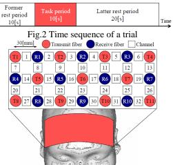
Fig.3 Optical fibers and channels
