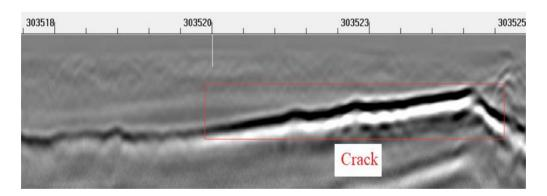
Figure 3. GPR image of tunnel ejection
