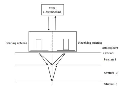
Figure 2. Principles of geological radar detection
