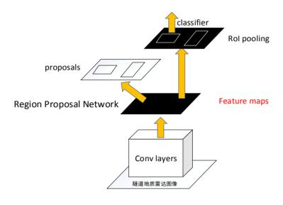
Figure 4. Structure chart Faster RCNN
