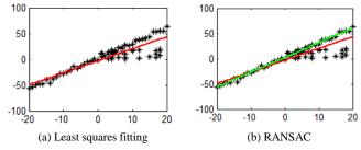
Figure 4. Comparison of Least Squares Fitting and RANSAC
