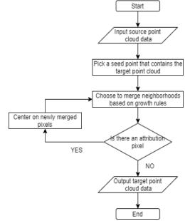
Figure 2. Area-based methods flow chart
