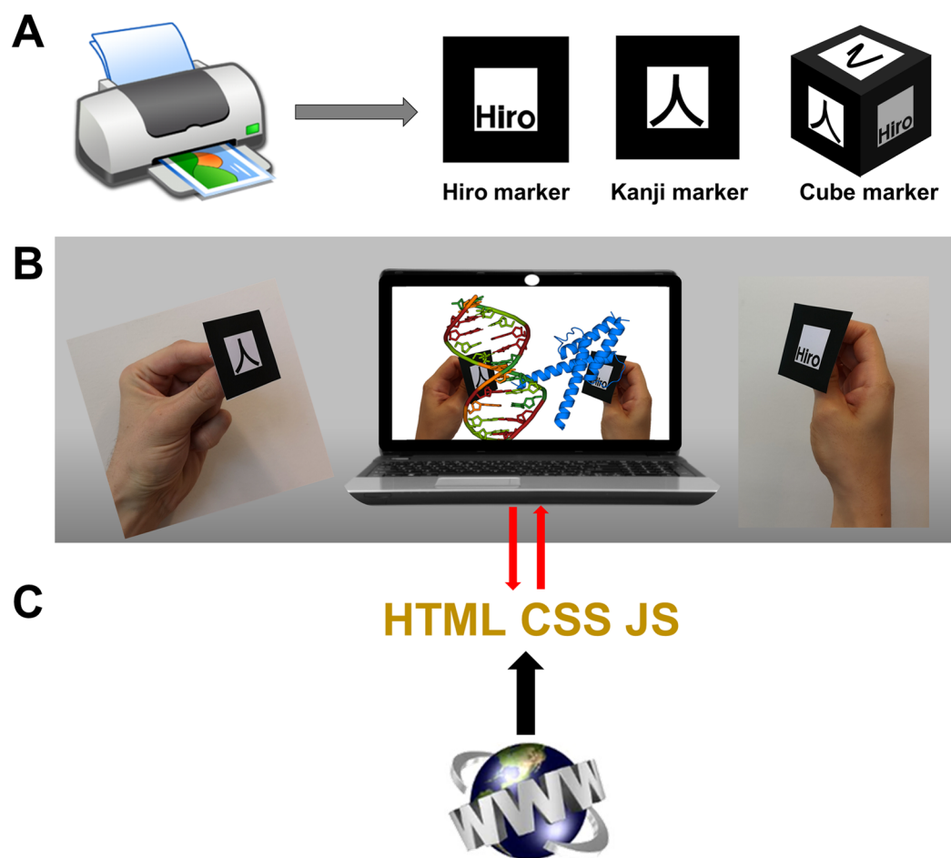
Figure 1 Commodity augmented reality in web browsers. (A) AR markers “Hiro” and “Kanji” are built into AR.js and its A-Frame wrap. Figure S1 shows them ready to print at various sizes. Custom markers including cube markers are also implementable. (B) In the proposed web apps the AR library feeds coordinate information to the graphics libraries and other algorithms. (C) The web pages must be hosted in servers compatible with the https protocol, but their content then runs exclusively on the computer.
