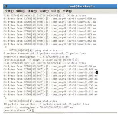
Figure 4. The ping implementation of the decimal network IPV9 address
