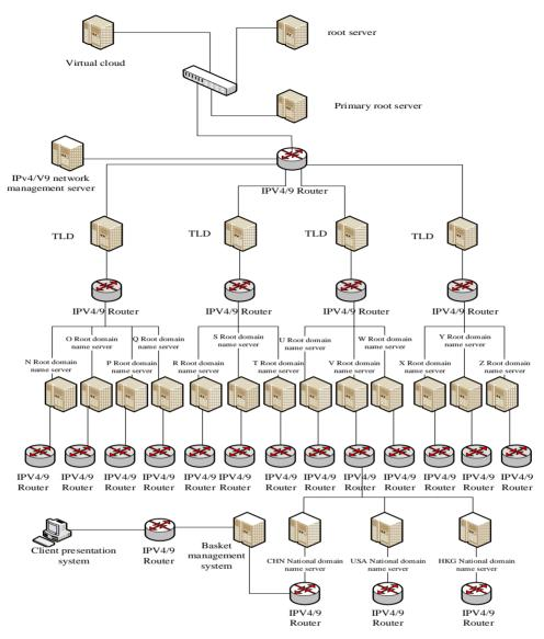
Figure 3. The IPV9 root name server system
