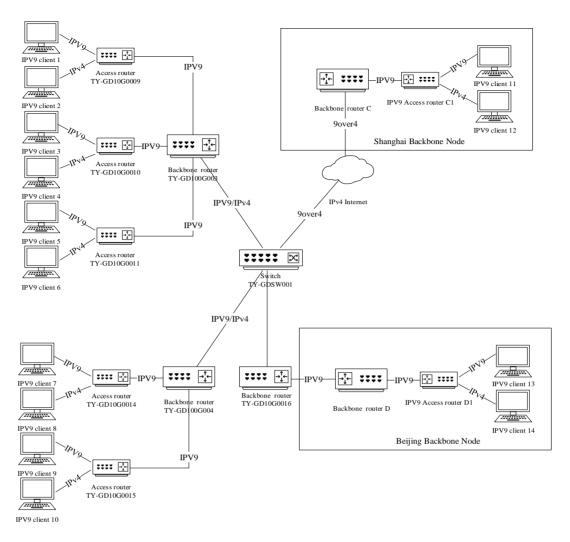
Figure 10. IPV9 hybrid network architecture test topology
