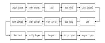
Figure 1. Multi-view image network structure diagram
