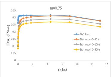
Figure 7. Validation of cross model with experimental data.
