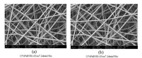
Figure 2. Nanofiber using PHD 4400 Syringe Pump at 30 kV (a) 10,000 times magnification, (b) 50,000 times magnification
