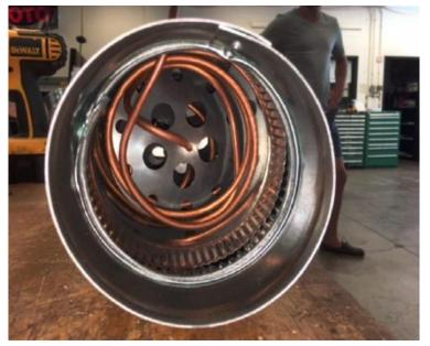
Figure 2. The heat exchanger prototype
