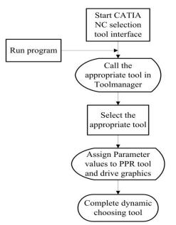
Fig.1. Tool library integrated solution.
