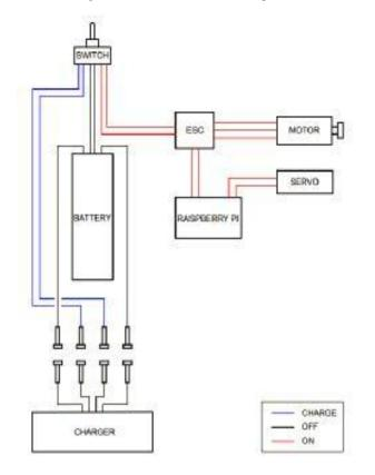
Figure 6. Layout of the Electrical Circuit
