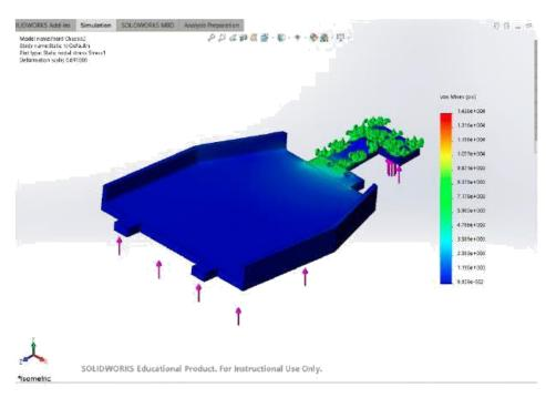
Figure 3. Chassis Fixed at Front Differential (Von Mises)
