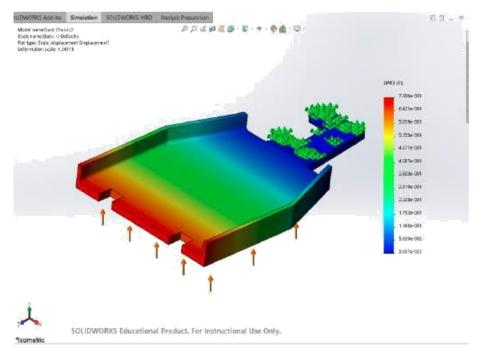
Figure 2. Chassis Fixed at Rear Differential (Displacement)
