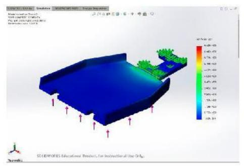
Figure 1. Chassis Fixed at Rear Differential (Von Mises)
