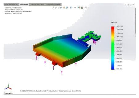
Figure 4. Chassis Fixed at front Differential (Displacement)
