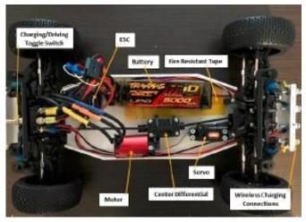
Figure 5. Detailed Picture of all Components
