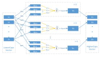
Figure 3. Dynamic routing algorithm
