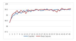
Figure 8. Comparison between the accuracy of capsule network and deep capsule network
