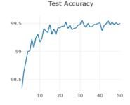
Figure 4. Test precision chart of capsule network under 50 epochs
