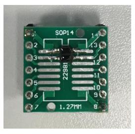
Figure 7. The optical sensor with adaptor
