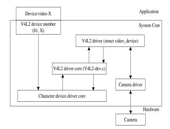
Figure 4. The structure of V4L2
