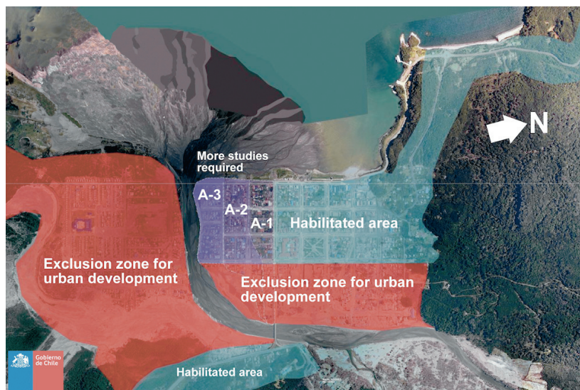
Fig. 2. Analysis of exposed areas and their categorization (Based on CIMM T&S Consultores, 2010, Municipalidad de Chaitén, 2011)
