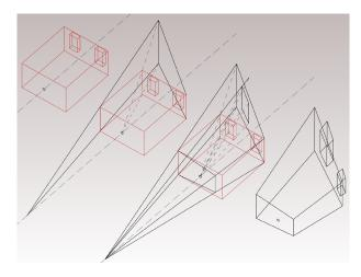
Fig. 6. Fig. 6. Projective construction of the Ames room model.
