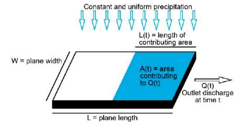
**Figure 2.** Conceptual overland homogeneous plane used for the conceptual formulation of the Rational Method.
