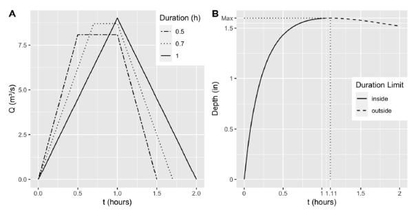
**Figure 3.** (**A**) Hydrographs resulting from the application of the Fort Wayne ID with the Rational Method for rainfall durations  $t_d$  equal to and 0.5, 0.7 and 1 h and  $t_c = 1$  h. (**B**) Depth Duration (DD) graph of the Fort Wayne ID equation. In both graphs, the ID equation is for  $T_r = 10$  years.
