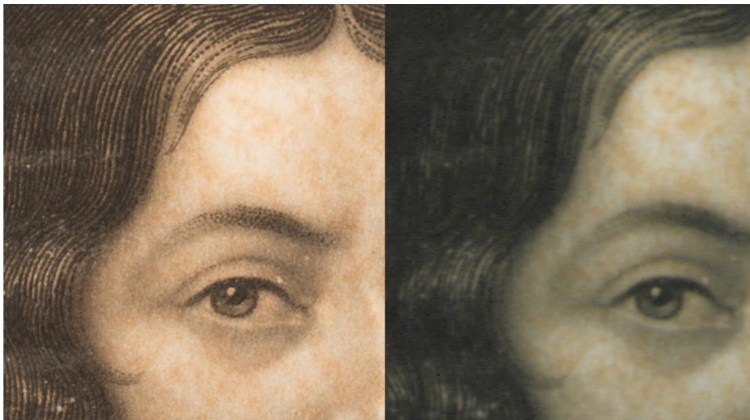
Figure 2. Comparative Images from DSLR (Left) and Overhead Scanner (Right), at 200 Percent Zoom. Image from Samuel M. Janney, The Life of William Penn; with Selections from His
