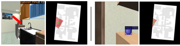
Figure 4: Qualitative result of the proposed method. Left: the object detection module was unable to detect the goal object (the mug, as indicated by the red arrow) when the agent is far from the object. Right: our proposed probabilistic map learns that the mug can be usually found on a cabinet, thus leads the agent to take a closer look at the cabinet and successfully find it.
