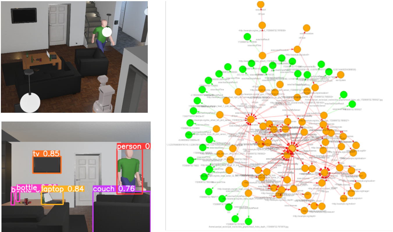
Figure 2: An example of the simulation environment (top left), the annotated view of the robot (bottom left), and the resulting observation graph when aggregated with the additional sensory data (right).
