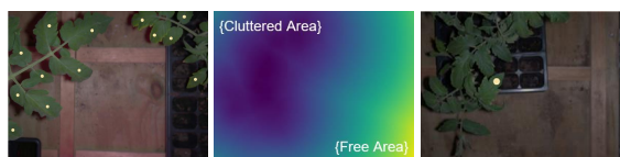
Figure 3: Top view image of the plants with grasp point per leaf (left), SDF of the workspace highlighting free vs occupied (center), optimal leaf and grasp point (right).
