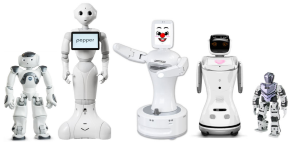
Figure 1: Humanoid robots are used to treat ADHD. NAO, Pepper, Silbot, Sanbot Elf, and Bioloid. are pictured from left to right.
