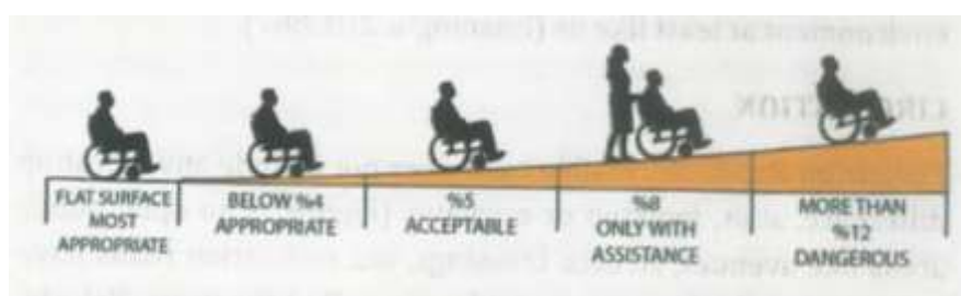
Fig. 6 (b) Ramp design specifications. Showing a variety of gradients appropriate for different ground or floor slopes. (Source: Yilmaz, 2018)
