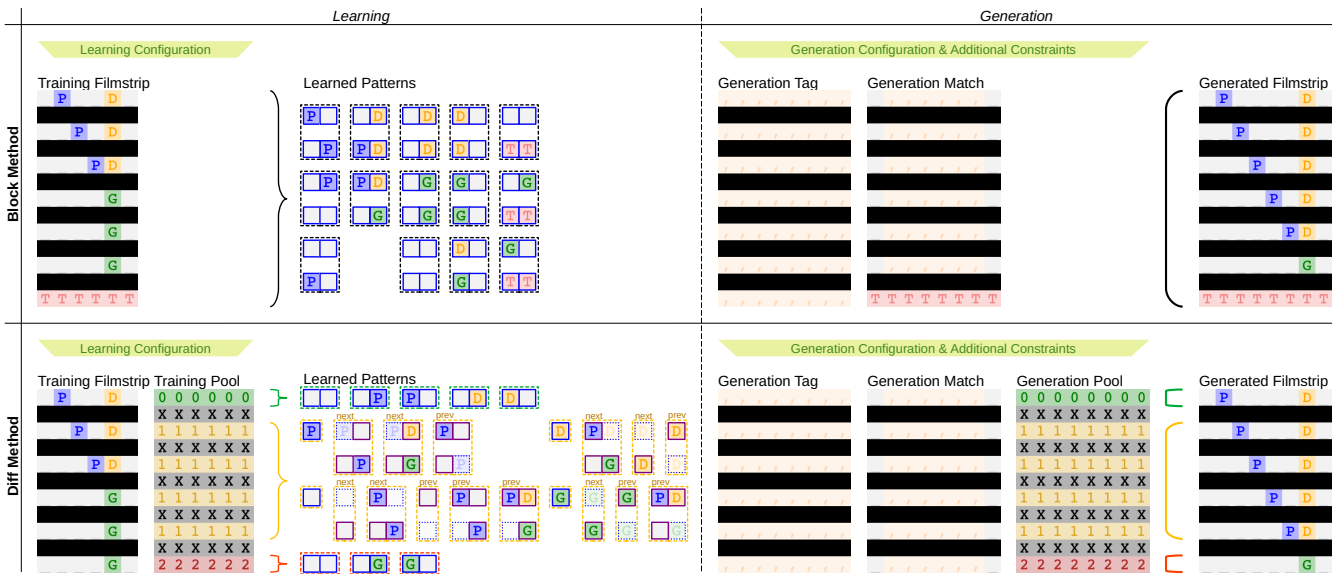
Figure 2: Overview of applying the block and diff methods on the simple demonstration game. In the learning process, given the training filmstrip, patterns are learned. Input-only patterns show tiles with solid blue outlines; input-output patterns show the input tiles lighter with dotted blue outlines and output tiles with solid purple outlines. In the generation process, learned patterns are applied to generate a new filmstrip of a longer level.
