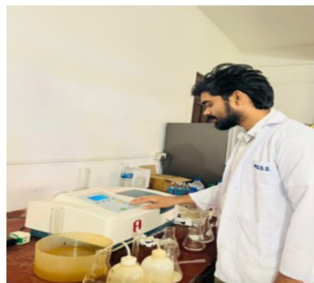
Figure 8: Measurement of absorbance using UV visible spectroscopy
