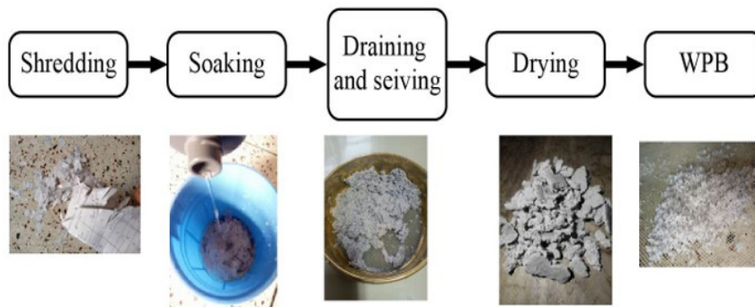
Figure 2: Schematic of Procedure for making WPB (waste paper binder)
