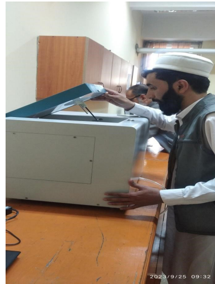
Figure 4: Automatic calorimeter machine for determining the thermal quality of coal
