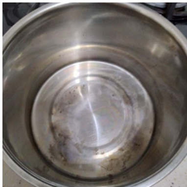
Figure 12: Stainless steel pot after the treatment of the lime scale with PGP stainless-steel pot
