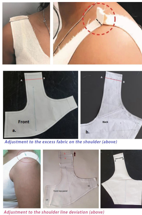
Figure 5: Excess fabric on shoulder and pattern correction (in caption blue), shoulder line deviation and pattern corrections (in caption red)
